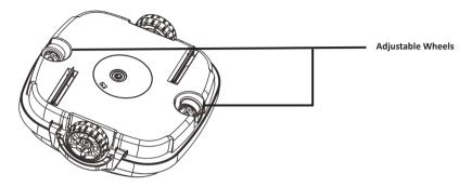
2. To adjust the wheel, open the lock buckles and remove the top cover. Locate the 2 adjustable wheels. Detach the wheel by pushing the wheel stem catch. Select the correct combination and insert the wheel until the catch clicks.
